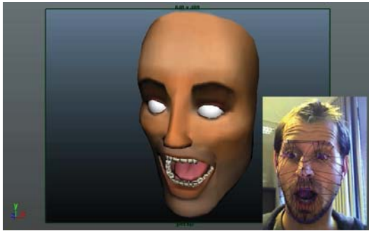
Figure 4: Realtime expression retargeting in Maya. The animation of the face model was driven by a motion capture device using realtime tracking of a web camera video.
