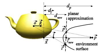
Figure 3. Iterative refinement of the ray parameter assuming that the environment is planar between points  $\vec{p}'$  and  $\vec{l}'$  corresponding to overshooting point  $\vec{p}$  and undershooting point  $\vec{l}$ , respectively.
