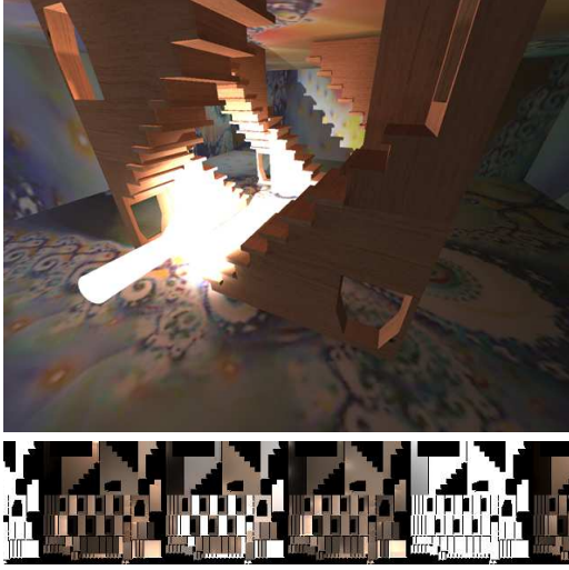
Figure 2: A few tiles of an LPM texture used to render the image above. Illumination corresponding to clusters of entry points is stored in tiled atlases.
