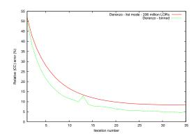
**Figure 7:** *The relative (CC) error in function of the iteration number*
