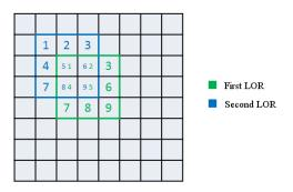
**Figure 6:** No memory conflict occurs if the two LORs intersect the slice in different voxels. The TOR width is 3 voxels and volumeDim = [8, 8, 8]. The numbers in the table show how the double for-loop iterates through the TOR-slice intersection.
