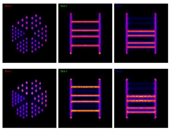
Figure 8: The binned (up) and the list mode (down) reconstruction's result, slices in the x, y and z direction.
