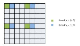
**Figure 4:** Loading one slice if volumeDim = [8, 8, 8] and blockDim = [4, 4].
