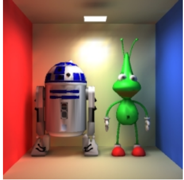
Figure 5: R2D2 meets an alien in the Cornell-box. The image was rendered with the new method using the biased variance reduction and the constant radiance step.
