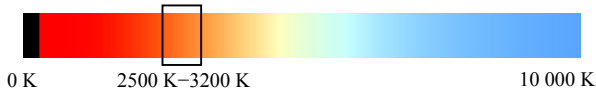
Figure 11: Black-body radiator colors from 0^{\circ}K to 10000^{\circ}K . Fire particles belong to temperature values from 2500^{\circ}K to 3200^{\circ}K .
