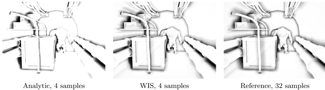
Fig. 10: Effects of the proposed weighted importance sampling (WIS). Note that the image rendered with weighted importance sampling from 4 samples is much closer to the reference image generated from 32 samples.
