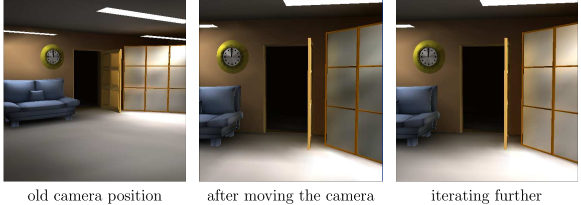
Figure 7.2: The left and right images show two frames of a walkthrough animation. The middle image is not seen by the user, but demonstrates the effect of just changing the camera location but not allowing time for the iteration to adapt to the new situation. Note that the algorithm needed a few iterations to correct the highlights.
