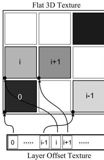
Figure 2.8: A 1D offset texture is used to easily address the origin of an arbitrary layer in the flat 3D texture.
