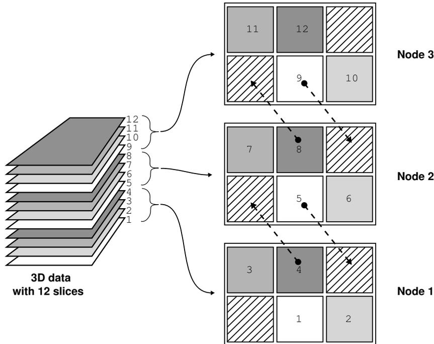
Figure 3.2: Data communication between the nodes of the cluster.
