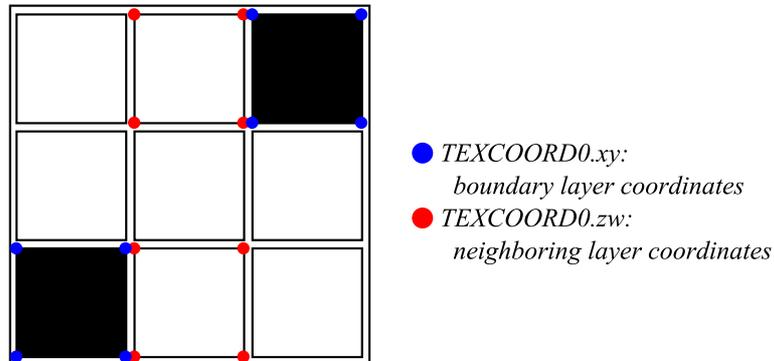
Figure 2.6: Texture coordinate setup of a quad for boundary layers.
