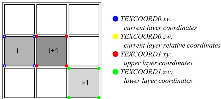
Figure 2.5: Texture coordinate setup of a quad for an inner layer.
