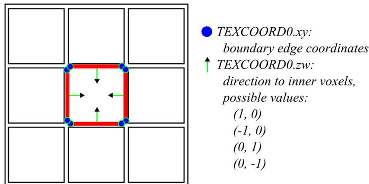
Figure 2.7: Texture coordinate setup of a line for a boundary edge.
