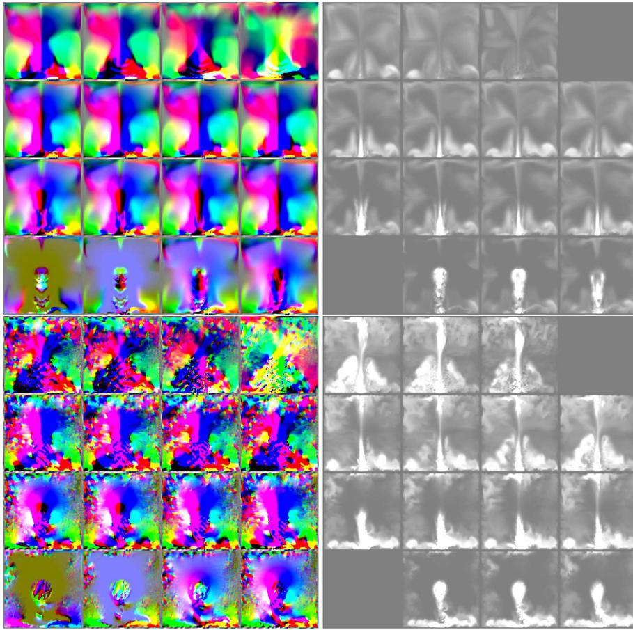
Figure 2.2: Flat 3D velocity (right column) and density (left column) textures of a simulation. The top row shows the simulation without, the bottom row with vorticity confinement.
