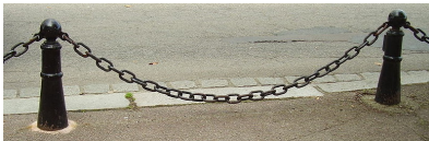
A hanging chain showing a catenary curve.
