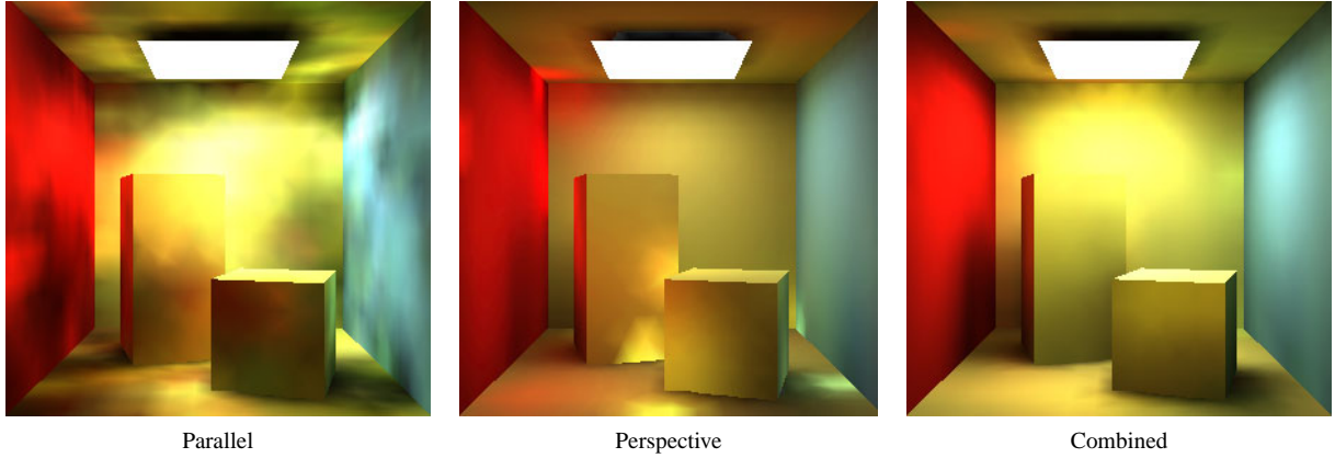
Figure 3: Comparison of stochastic iteration using parallel (left), perspective (middle) ray-bundles and the combination of the two methods (right) using the same computation time (5 secs)
