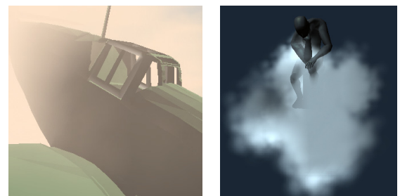
Figure 4: Volume rendered with depth impostors eliminating billboard clipping artifacts
